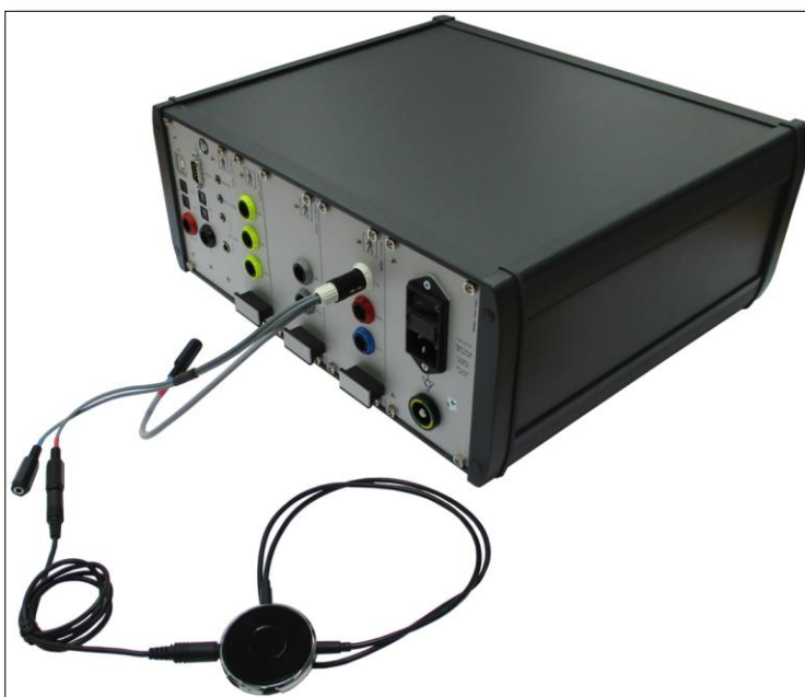
Figure292: Setup with the audiometer and cable connection to the SAMBA 2 G streamer
