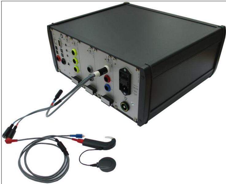
Figure291: Setup with the audiometer and direct cable feed into the SONNET CI processor
